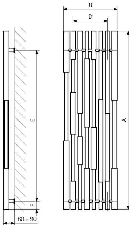
A — Height B — Width C1-C5 — Distance between pipe centres D — Horizontal distance between mounting bracket centres
