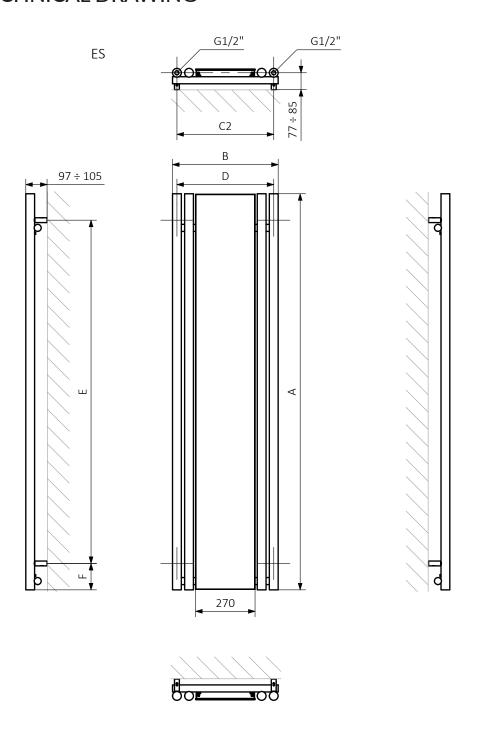
$A-Height\ B-Width\ D-Horizontal\ distance\ between\ mounting\ bracket\ centres\ E-Vertical\ distance\ between\ mounting\ bracket\ soft the\ radiator$
