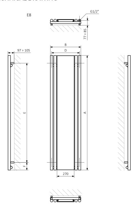
$A-Height\ B-Width\ D-Horizontal\ distance\ between\ mounting\ bracket\ centres\ E-Vertical\ distance\ between\ mounting\ bracket\ soft the\ radiator$
