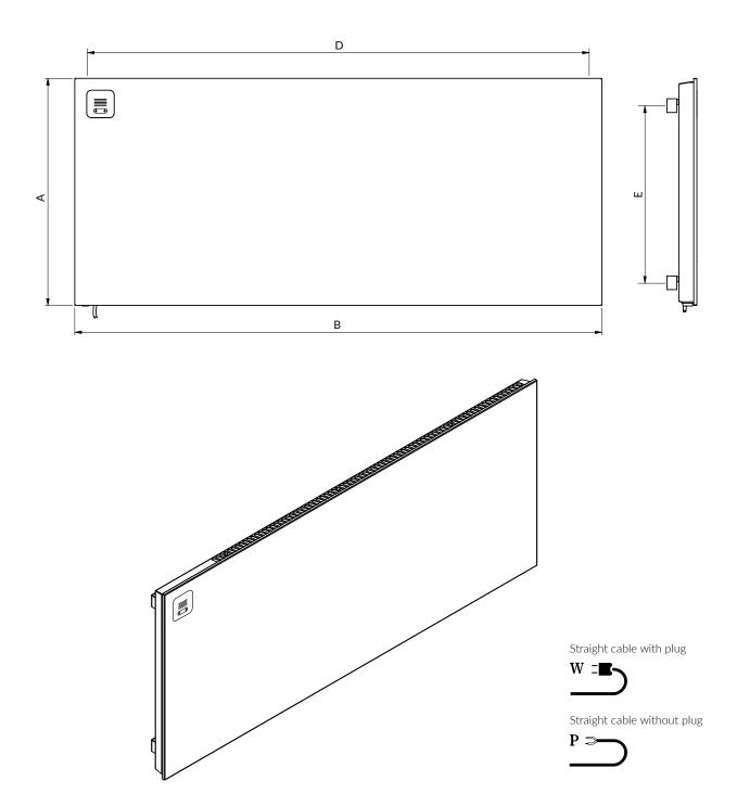
$A-Height\ B-Width\ D-Horizontal$  distance between mounting bracket centres  $\ E-Vertical$  distance between mounting brackets
