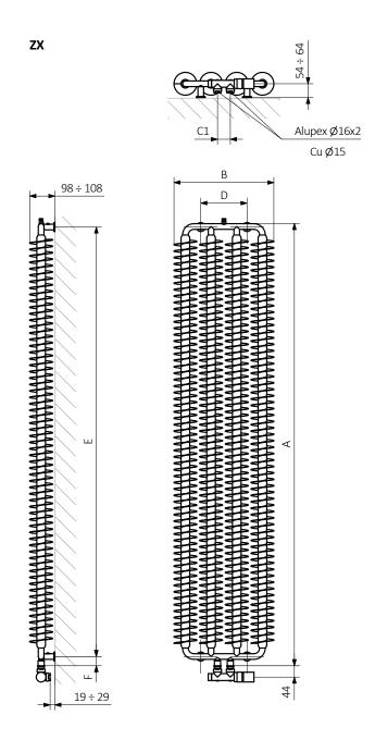
$A- Height \quad B- Width \quad C1-C5- Distance \ between \ pipe \ centres \quad D- Horizontal \ distance \ between \ mounting \ bracket \ centres \\ E- Vertical \ distance \ between \ mounting \ brackets \quad F- Distance \ between \ a \ mounting \ bracket \ and \ the \ bottom \ of \ the \ radiator$
