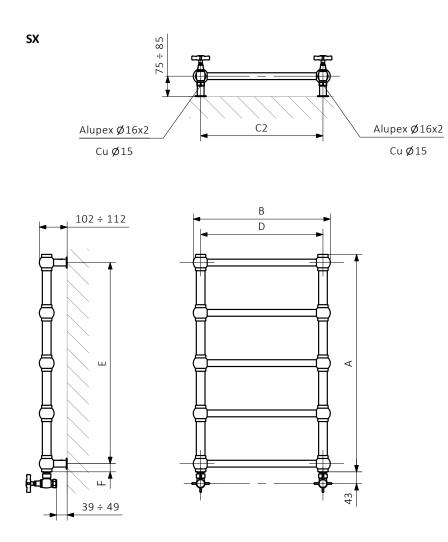
$\begin{array}{lll} A-Height & B-Width & C1-C5-Distance between pipe centres & D-Horizontal distance between mounting bracket centres \\ E-Vertical distance between mounting brackets & F-Distance between a mounting bracket and the bottom of the radiator \\ \end{array}$
