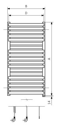
$A- Height \quad B- Width \quad C1- C5- Distance \ between \ pipe \ centres \quad D- Horizontal \ distance \ between \ mounting \ bracket \ centres \\ E- Vertical \ distance \ between \ mounting \ brackets \quad F- Distance \ between \ a \ mounting \ bracket \ and \ the \ bottom \ of \ the \ radiator$
